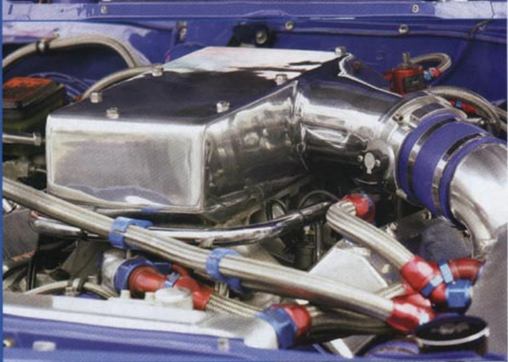
TOP: Prepare to drool! Originally a SL, Gerald has taken the capacity out to 5.7L, fitted forged internals, 2000hp-capable Vortech, custom cooler and plenum and wired in a MoTeC M800 brain resulting in a crazy 567kW at the treads
